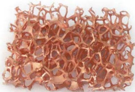
Copper foam, now available from Goodfellow, combines the outstanding thermal conductivity of copper with the structural benefits of a metal foam. These features are of particular interest to design engineers working in the fields of medical products and devices, defence systems and manned flight, power generation, and the manufacture of semiconductor devices.
