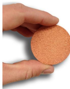
*New microporous copper foam, with a relative density of around 37% and a very large surface area, is a powerful heat sink.*
